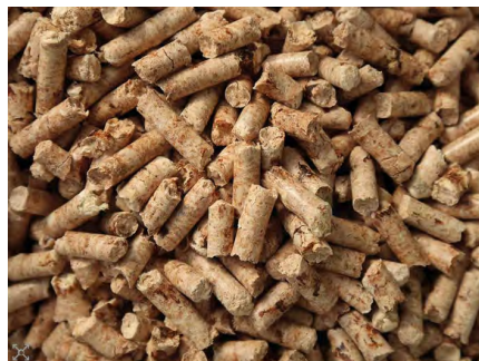
Fig. 8. Energy form: UK biomass plants use wood pellets of leftover material from managed forests (Source: Ravilious, 2020)
