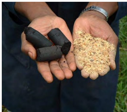
Fig. 13. Torrefied biomass is shaped into briquettes in Nairobi, Kenya (Source: The National Renewable Energy Laboratory <NREL> Photograph courtesy, Chardust LTD, Biomass Energy, 2022)
