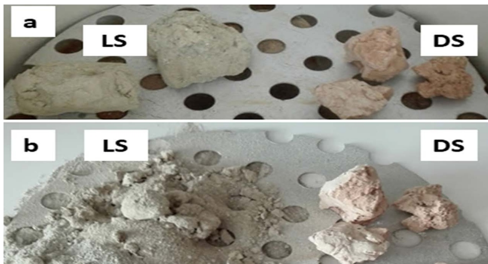
Phot. 2. Lumps of washing aggregates sludges a – after firing, b – after 4 hours of steam subjection; DS – fired lumps of dolomite sludge, LS – fired lumps of limestone sludge – LS
