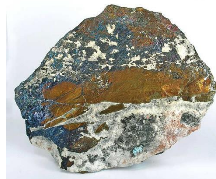
Ore of covellite (blue) and of chalcopyrite (brown)
