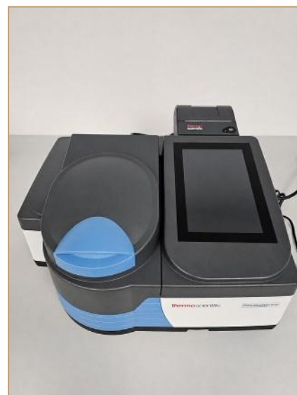
Spektrometr UV-Vis Aquamate 8100 (Thermo Scientific)
